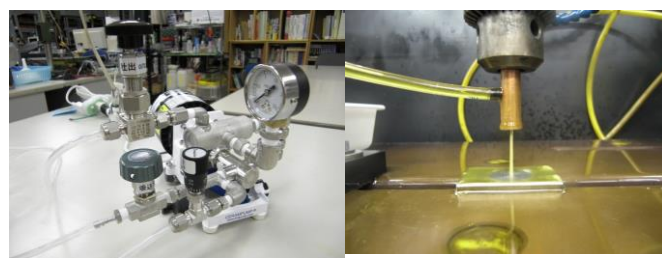
Fig.1 The micro bubble pump and the electrode
