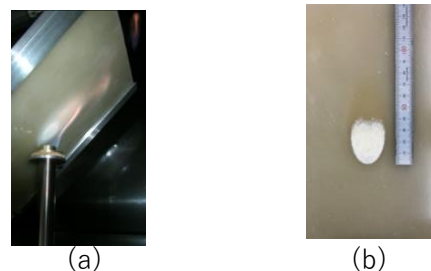
Fig. 4 Observation images of test specimen during (a) and after (b). combustion test.
