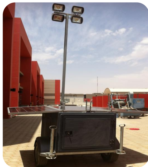
Fig.2 Mobile solar lighting tower
